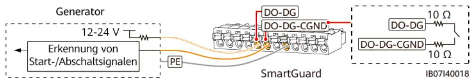
**Abbildung E-2** Generator-Alarmsignal
