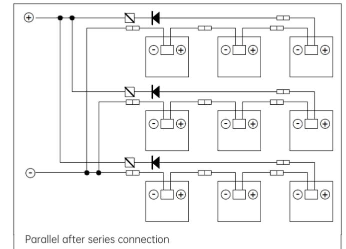
If the PV module is passed through by a reverse current greater than the maximum fuse current of the PV module, the PV module shall be protected with an over current protector of the same specification. If more than two strings are connected in parallel, each PV module string shall be protected with an over current protector as shown above.
